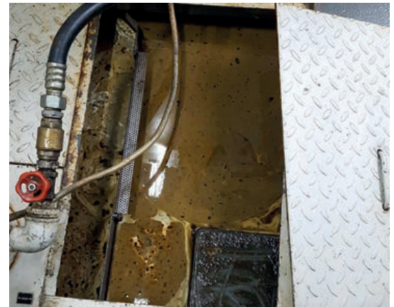
Without an effective filter: microparticles coat themselves with oil and float • uncontrolled segregation
