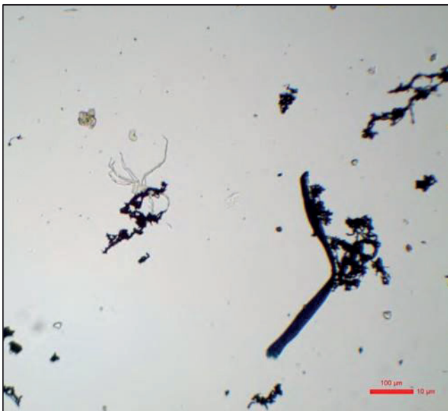
Cooling lubricant sample from ongoing large-scale production. Particle sizes well above the desired ones Tolerances and surface qualities, despite the band filter system!
