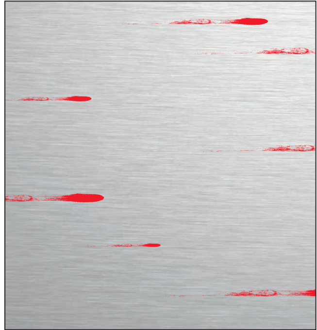
Suspensions and particles damage the surface and the grinding wheel
