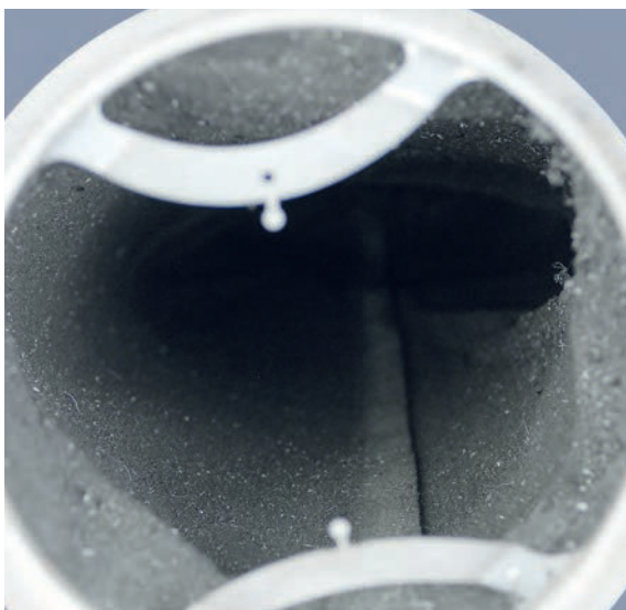
Chips and suspended matter from the filter on the path to the tool were intercepted
