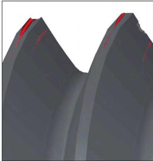
Damage pattern with high particle load, cutting edge fractures and damage to the tap due to jamming particles
